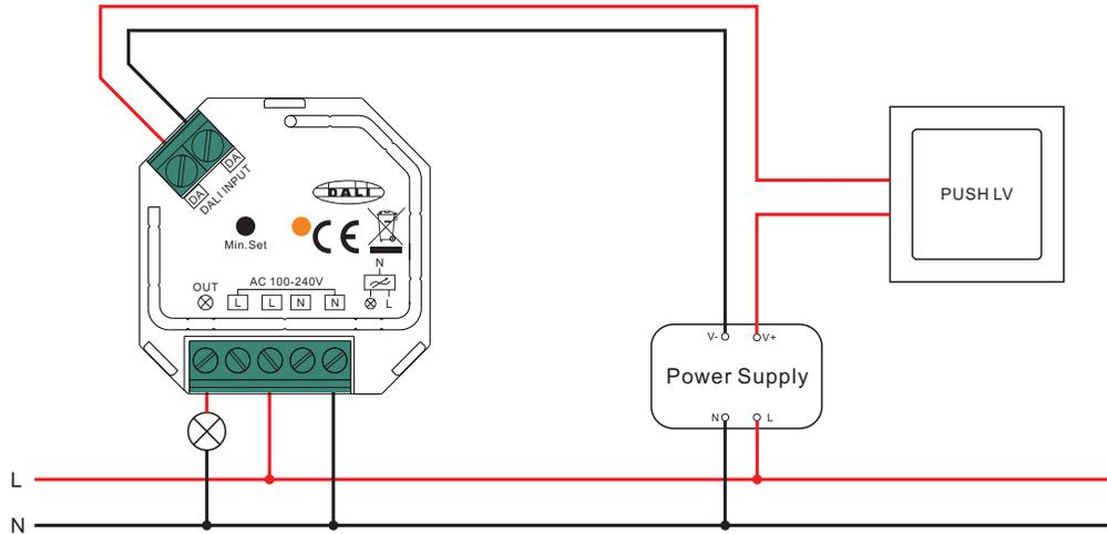
This phase dimmer adopts trailing edge dimming (reverse phase control), please make sure the connected loads support reverse phase control. Please refer to the user manual of the load or consult the supplier of the load.
