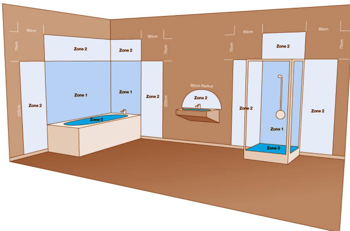
In addition to the above, if there is a likelihood of water jets being used for cleaning purpose in zones 1,2 and 3 a fitting rated a minimum IP65 must be used. Full details can be found in the latest copy of the IEE wiring regulations.
